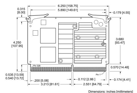
**Figure 7. CPU Module (Component Dimensions)**
